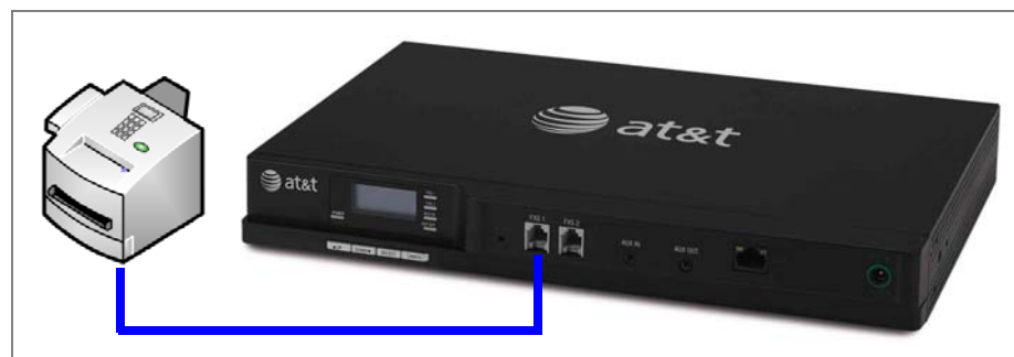
Figure 3. Fax Machine Connected to FXS Port
